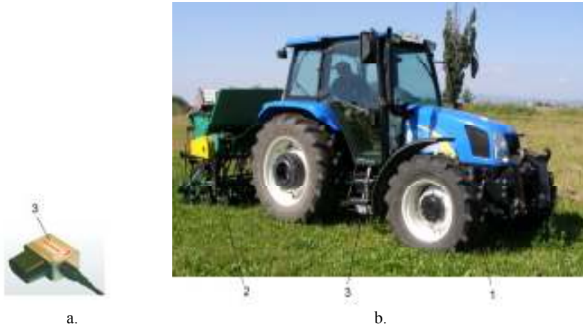
Figure 11. Optical speed transducers AQUA L 350 type (a) and transducer location on the tractor (b): 1-tractor New Holland tractor (TL 100 type); 2-oversowing machine (type) MSPD-2,5; 3-optical transducers of speed and displacement.
