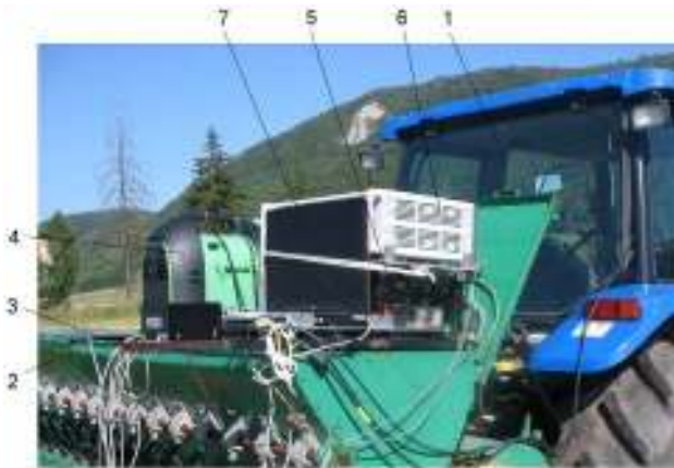
Figure 12. Location of measurement and data acquisition equipment on the system: 1-tractor; 2-grassland oversowing machine; 3-frame for location of measurement and data acquisition equipment; 4-power supply; 5- voltage stabilizer; 6- booster modular system (MGCplus); 7-laptop P4
