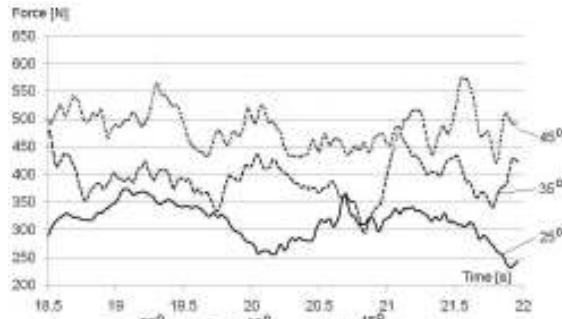
Figure 13. Section resistance force variation in time depending on the furrow attack angle.
