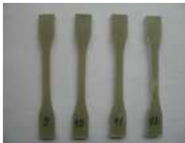
Figure 2: Samples 9-12 before being subjected to tensile
