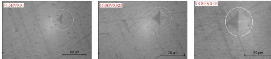
**Figure 2:** Indentations in human dentine for: 10gf/10s, 25gf/10s, 50gf/10s.
