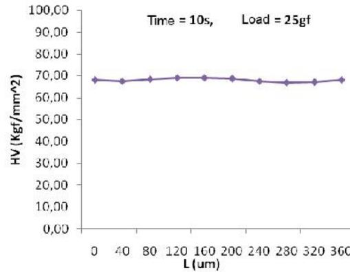
**Figure 3:** HV values on the measured length L, at 25gf/10s
