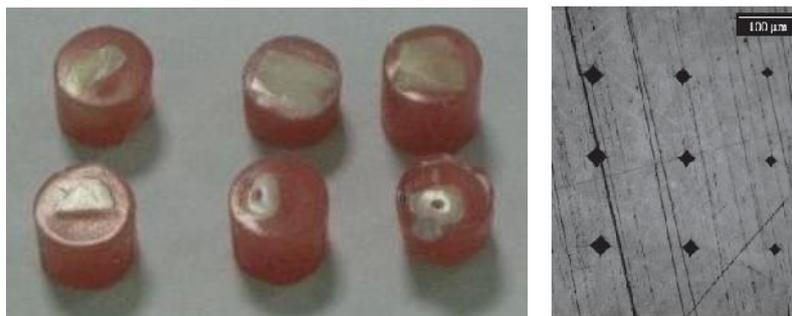
Figure 1: The dentine samples and a capture of the indentations
