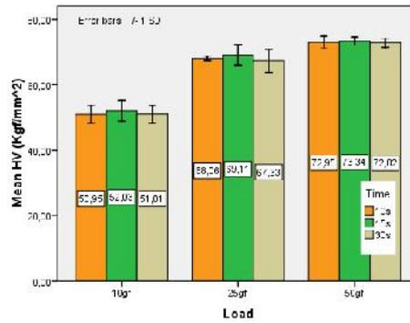
**Figure 5:** Comparison of the dentine HV values at a given load and different durations.
