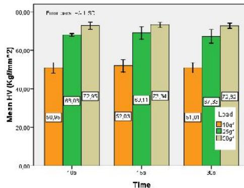
**Figure 5:** Comparison of the dentine HV values at a given duration and different loads.
