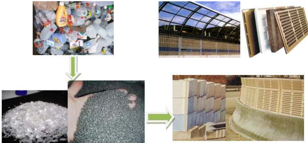
Figure 3. Recycling plastic and turning it in street barriers [1, 8, 10]
