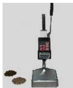
Figure 3: Maturity meter device 200
