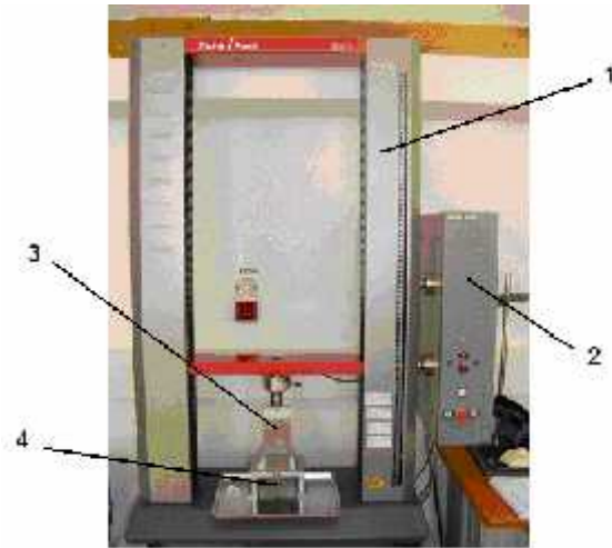
Figure 1: Zwick /Roell stand for cutting resistance determination
