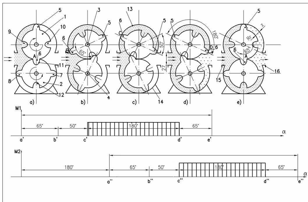
Fig. 1. The motor torque developed by the steam pressing on the rotating pistons (5) and (6) of the upper rotor (1)
