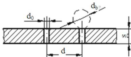
Fig. 2. Hole spacing in the FBG disk
