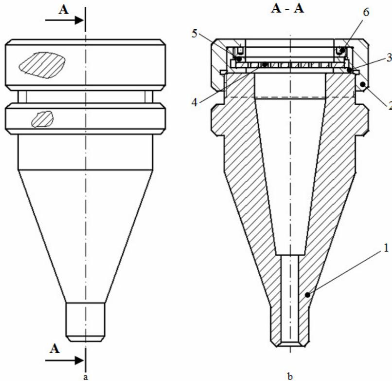
Fig. 1. The fine bubble generator a – front view; b – cross-section
