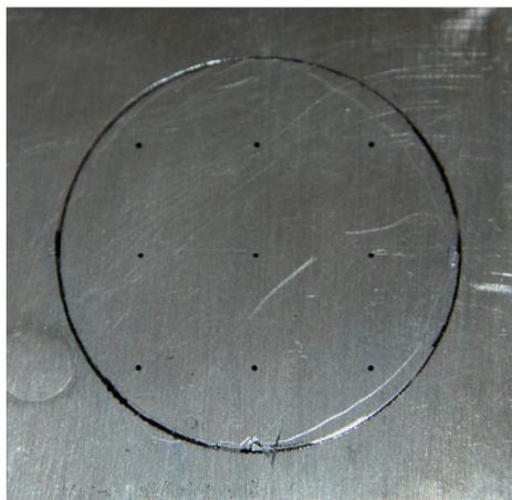
Fig. 5. Hole network, practiced by electro-erosion
