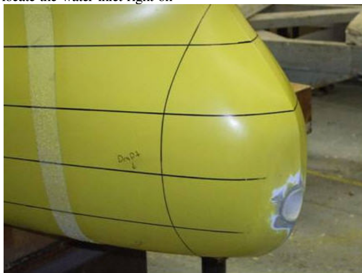
Fig. 3.3. Location of Forward Ballast Trunk Inlet
