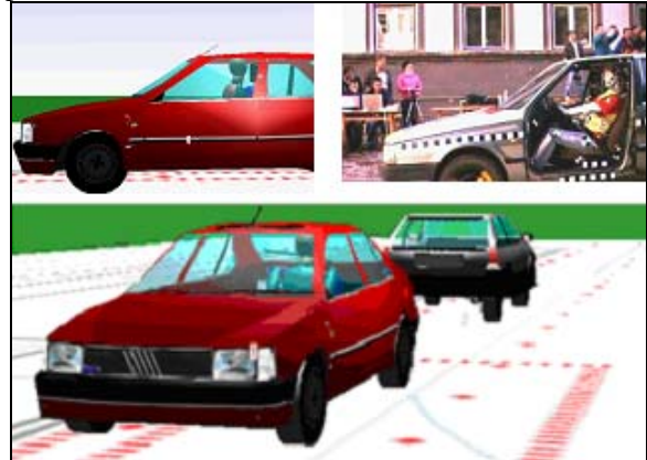
Fig. 2 Images of vehicle pushed, obtained from the PC-Crash and simulation video evidence of the experiment
