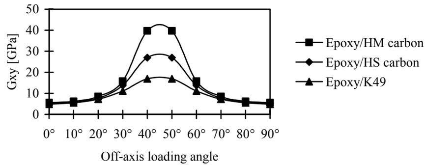
**Figure 5:**  $G_{xy}$  shear modulus for a [0/90/0/90] epoxy based composite laminate
