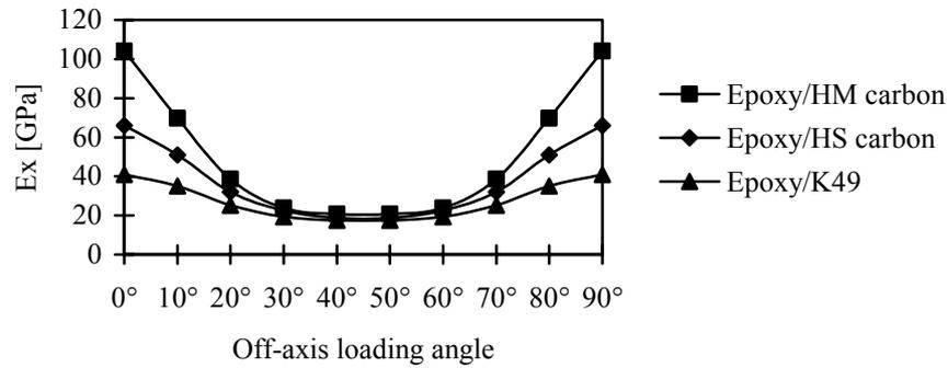
**Figure 4:**  $E_x$  Young modulus for a [0/90/0/90] epoxy based composite laminate
