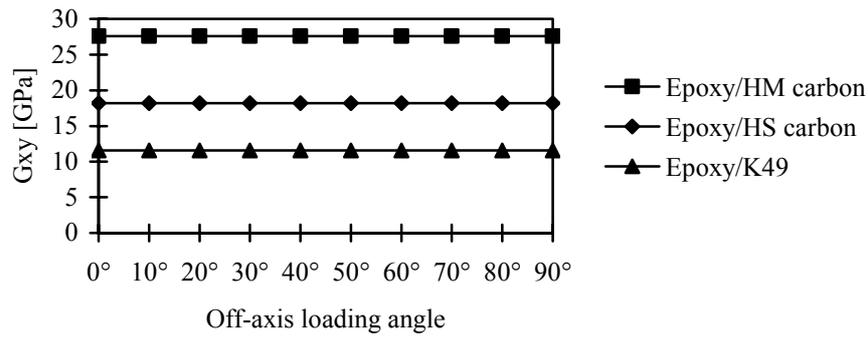
**Figure 8:**  $G_{xy}$  shear modulus for a [0/45/-45/90] epoxy based composite laminate
