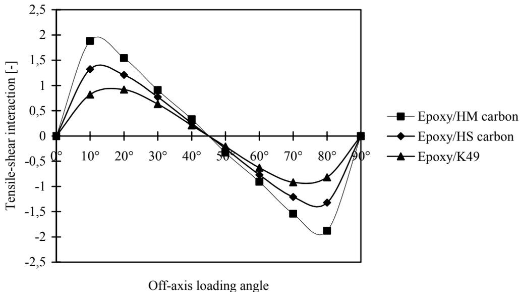
**Figure 13:** Distribution of tensile-shear interaction in a [0/90/0/90] composite laminate
