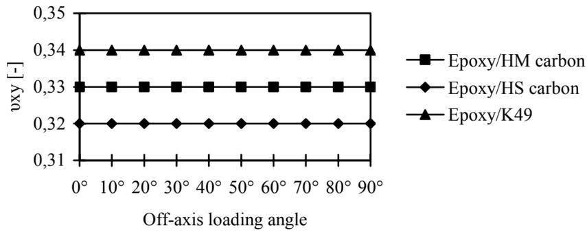
**Figure 9:**  $\nu_{xy}$  Poisson ratio for a [0/45/-45/90] epoxy based composite laminate
