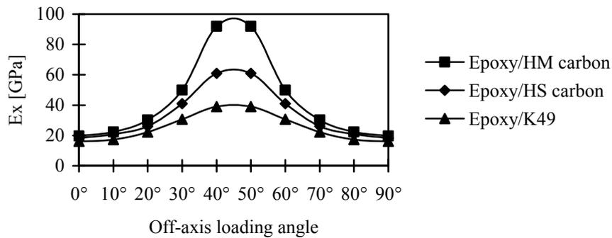
**Figure 10:**  $E_x$  Young modulus for a [45/-45/45/-45] epoxy based composite laminate
