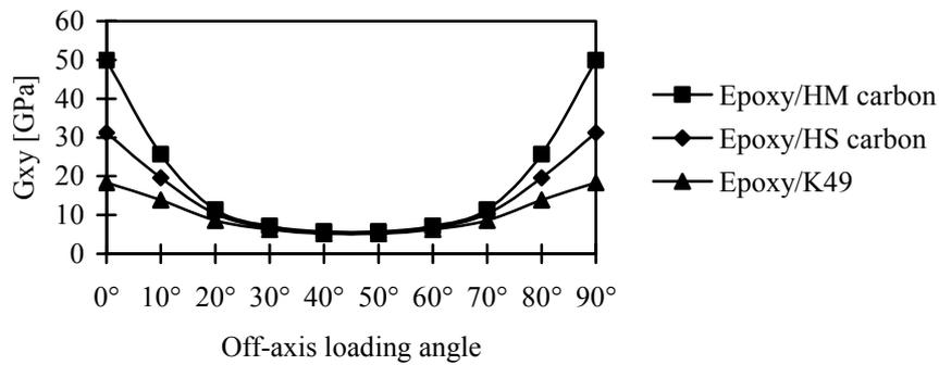
**Figure 11:**  $G_{xy}$  shear modulus for a [45/-45/45/-45] epoxy based composite laminate
