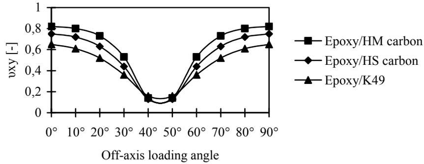
**Figure 12:**  $\nu_{xy}$  Poisson ratio for a [45/-45/45/-45] epoxy based composite laminate
