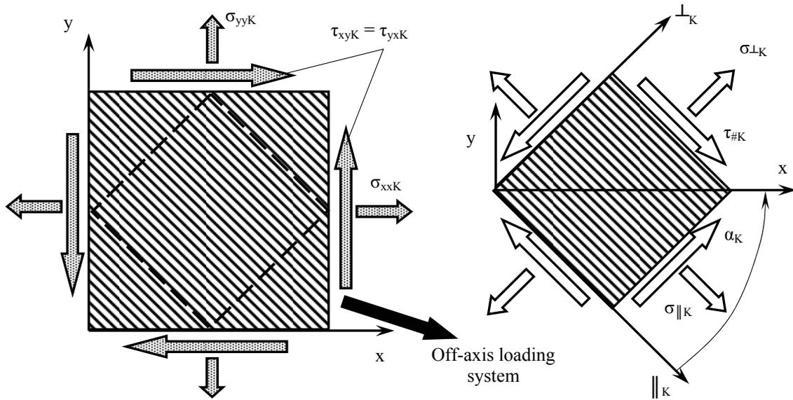
**Figure 2:** Loading scheme of a composite laminate
