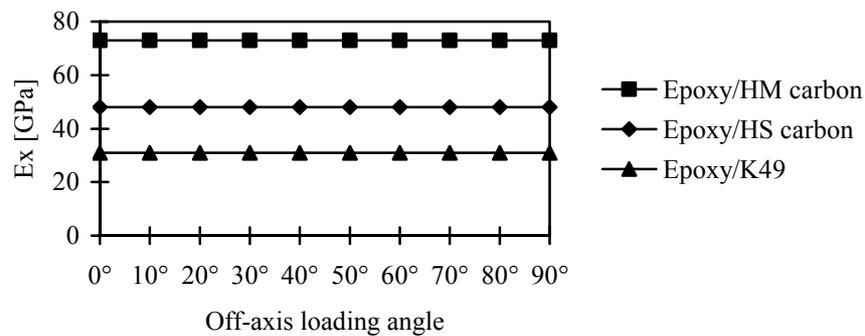
**Figure 7:**  $E_x$  Young modulus for a [0/45/-45/90] epoxy based composite laminate
