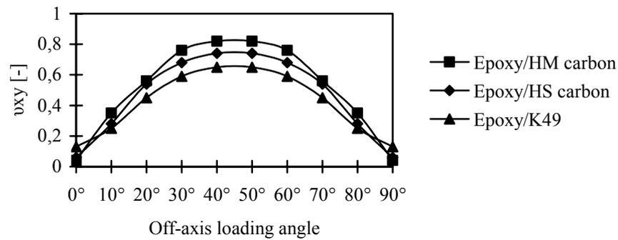
**Figure 6:**  $\nu_{xy}$  Poisson ratio for a [0/90/0/90] epoxy based composite laminate
