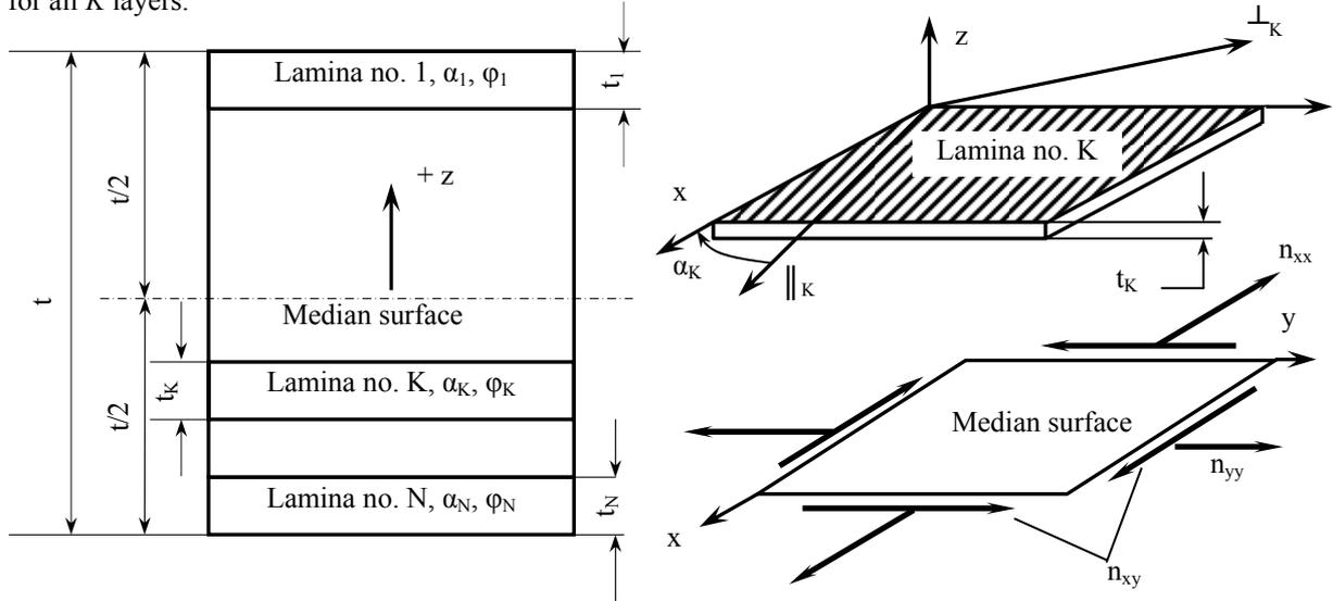
**Figure 1:** Constructive scheme of a composite laminate
