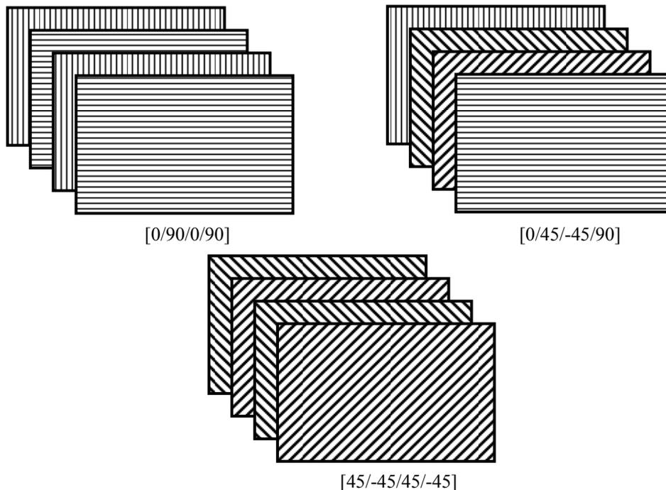
**Figure 3:** Architectures of some advanced composite laminates
