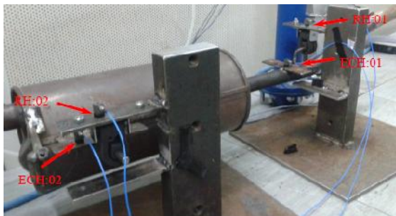
Figure 3: Exhaust line on rubber elements
