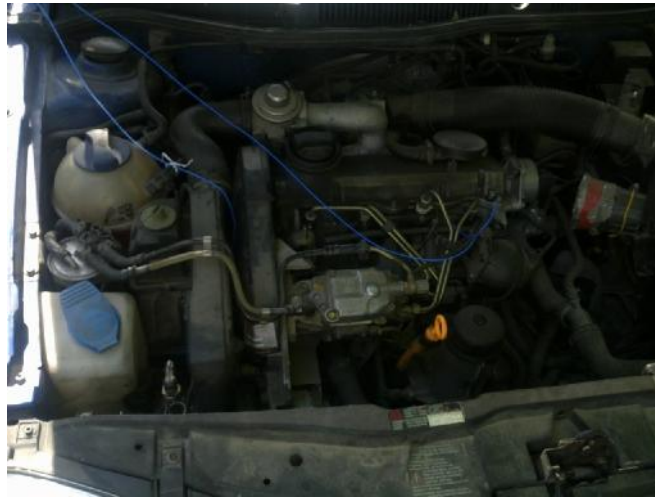
Figure 4. The montage of the two accelerometers on the engine mounting and on the valve train mechanism block
