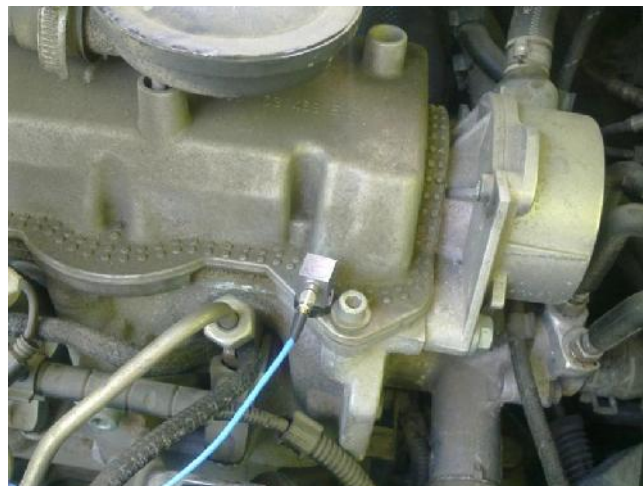
Figure 3. Accelerometer mounted on the valve train mechanism block
