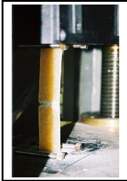
Figure 6. Failure mode in the center of the RT300 glass fiber-reinforced polyester specimens
