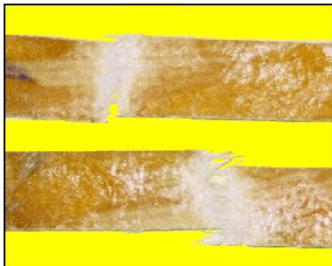
Figure 11. Broken glass fiber-reinforced HDPE composite specimens
