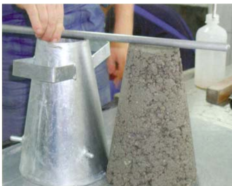
Fig. 3. Concrete consistency by slump test
