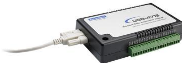
Fig. 5 Data acquisition board used for the test bench
