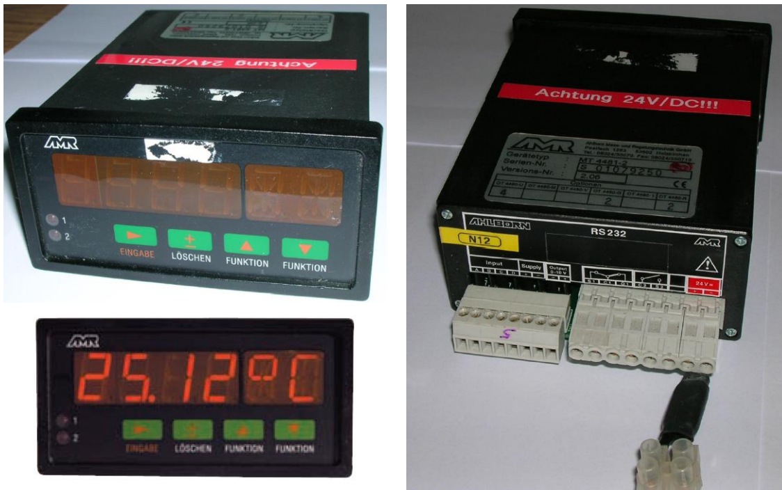
Fig. 4 AMR MT 4481-2 device used for the test bench
