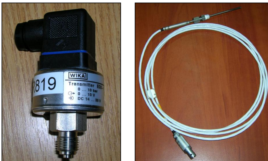
Fig. 3 Pressure and temperature sensos used for the test bench
