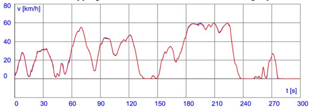
Figure 7: Plots of simultaneous speed records obtained with two similar GPS devices (Garmin GPS 18x-5Hz) placed very close one to other
