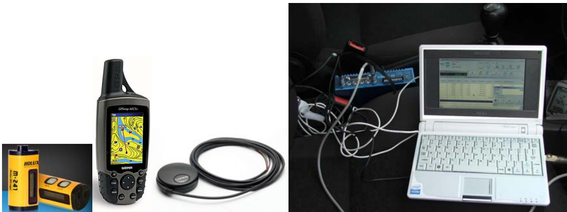
Figure 1: The GPS devices used in measurements: left – Holux M-241; middle left – Garmin GPSMap 60CSx; middle right – GPS 18x-5Hz; right – Racelogic VBox (the blue case) and the previous two devices
