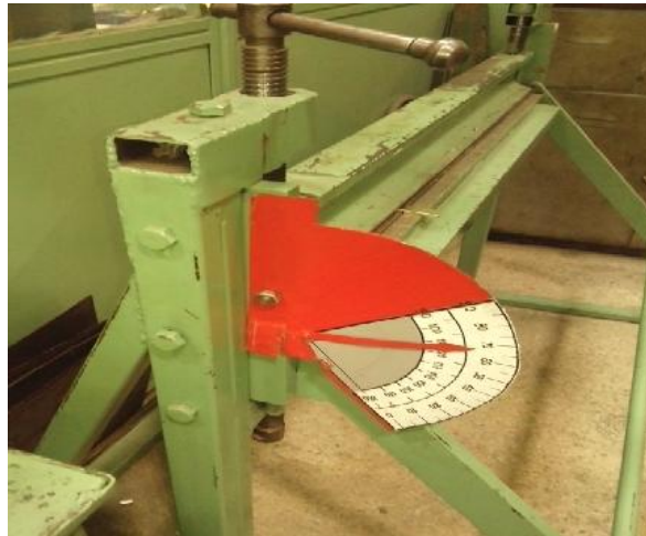
Figure 4: Free bending tests of technological samples using the AbKant 850 apparatus
