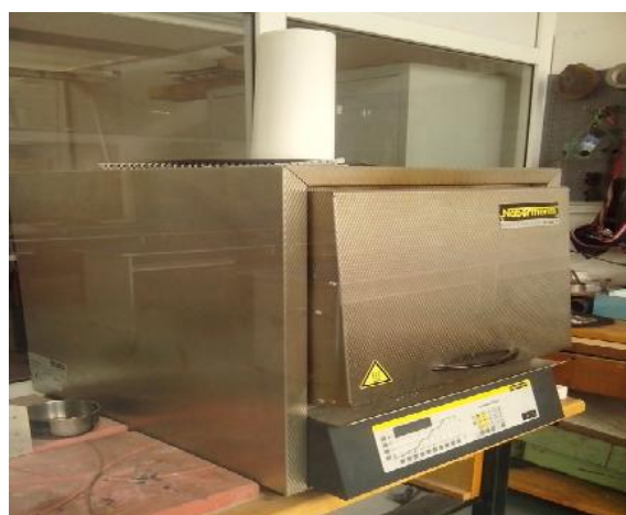
Figure 3: The oven for heating to demagnetize of technologic samples, model Nabertherm and temperature range 30-3000 0 C
