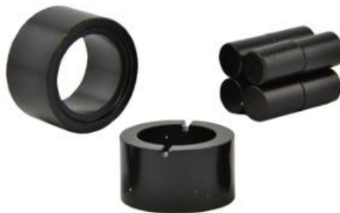
Figure 4: Technological tests composite permanent magnets, based on NdFeB, subjected to cutting machining
