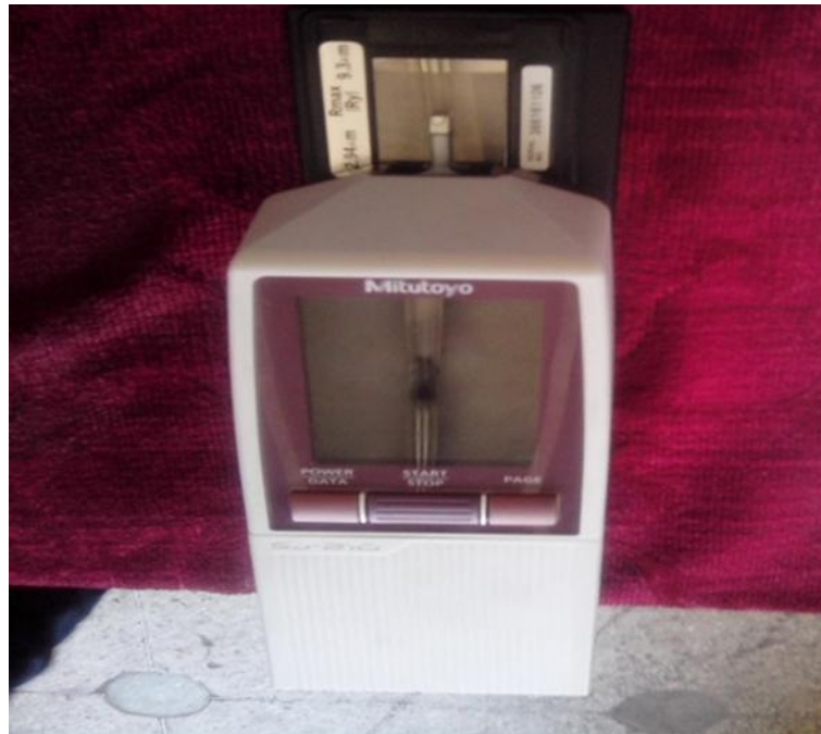
Figure 3: Roughness meter MITUTOYO-SJ-210 with diamond palpation element
