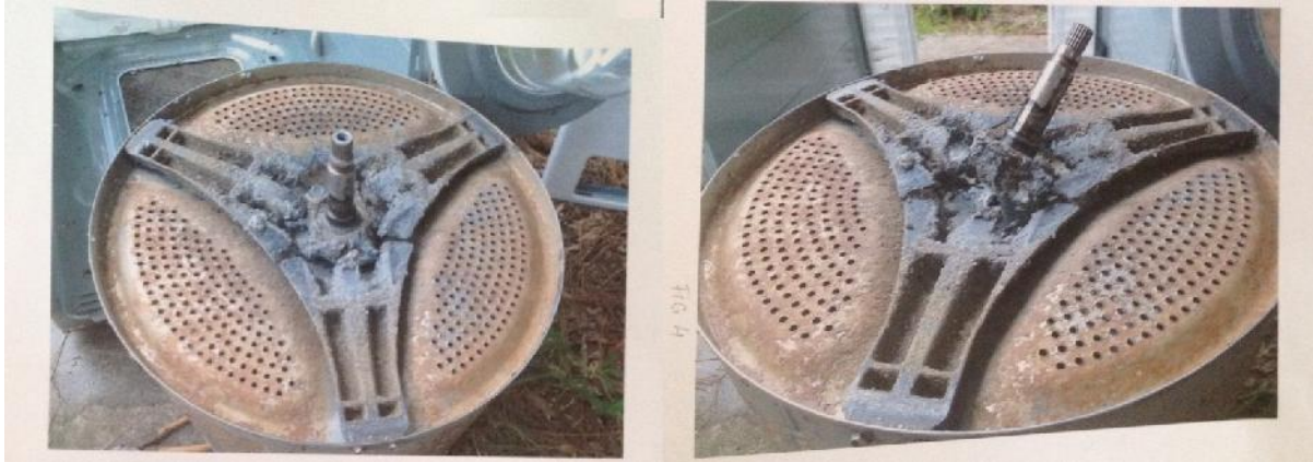
Figure 4: The fastening system of the drum with three branches deteriorated
