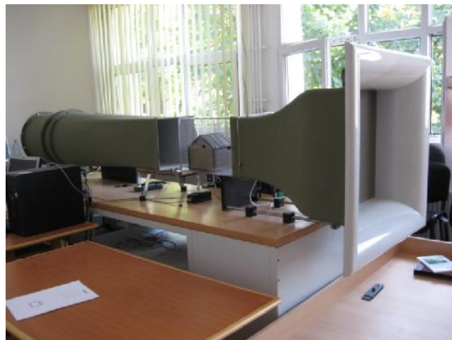
Figure 10. The wind tunnel with a greenhouse model located in a position of the airflow direction
