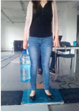
Figure 5: Positioning Kistler platform- subject for static weight measurement.
