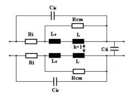
Fig. 13. Common mode choke
