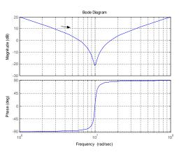
Fig. 9. Bode diagram of the behavior of a high frequency capacitor
