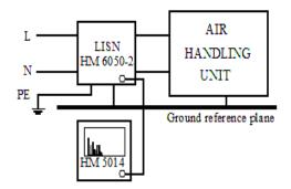
Fig. 2. The schematic test setup for conducted interference
