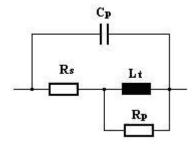
Fig. 10. Equivalent schematics of a high frequency inductor
