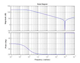
Fig. 7. Bode diagram of the behavior of a high frequency resistor
