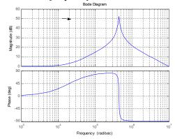
Fig. 11. Bode diagram of the behavior of a high frequency inductor
