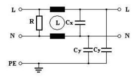
Fig. 5. Typical topology of mains filter
