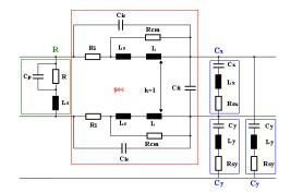
Fig. 14. Equivalent schematics of an EMI filtering cell
