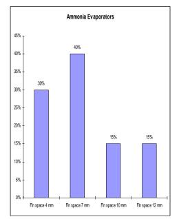
Fig. 3 Evaporators used in Roman<u>i</u>an ammonia refrigeration plants in the last four years
