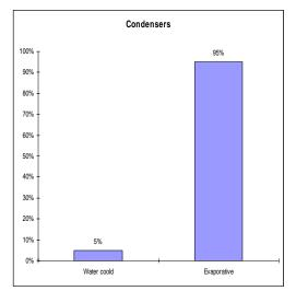
Fig. 4 Condensers used in Roman<u>i</u>an ammonia refrigeration plants in the last five years
