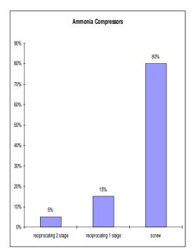
Fig 2 Compressors used in Romanian ammonia refrigeration plants in the last five years
