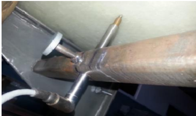
Figure 5: Displacement transducer LVDT
