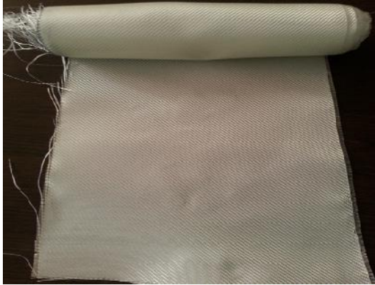
Figure 1: Twill fabric with thickness of 0.2mm
