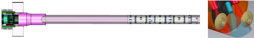
Figure 6: Representation of cutting with rollers in the middle and to end of pressure tube
