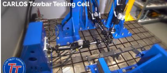
Figure 3: Towing assembly on the test bench
