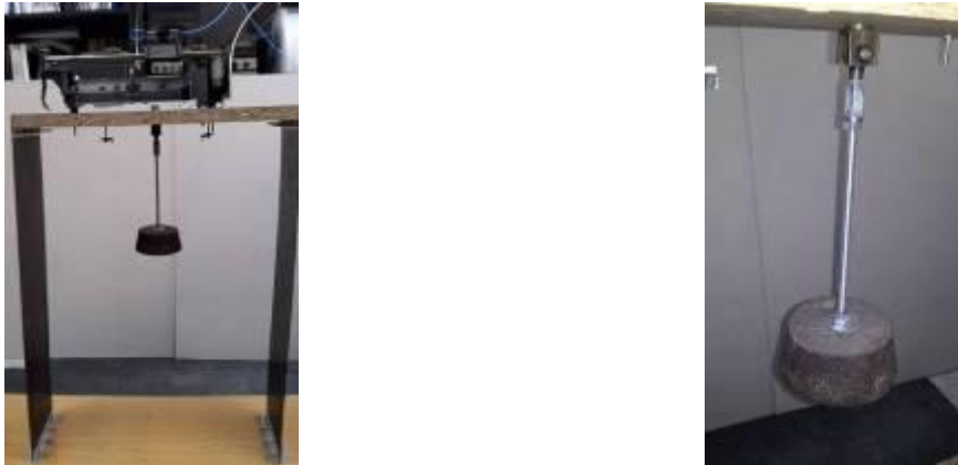
Figure 2: The constructive details of the structure and of the pendulum absorber system
