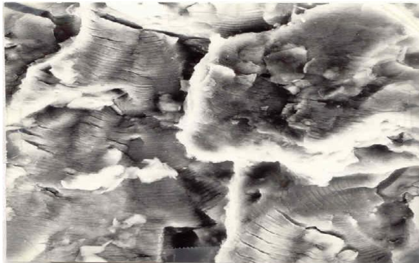
Figure 1a: A fatigue crack surface in Al-alloy
