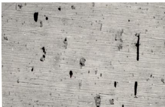
Figure 4: Microstructure of Al 6061 T651 (x300)
