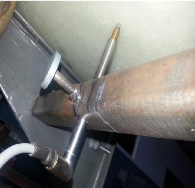
Figure 4: The location of Displacement transducer (LVDT)
