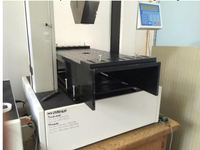
Figure 1: Table with adjustable clamping plates mounted on a “LS100 Plus” testing machine
