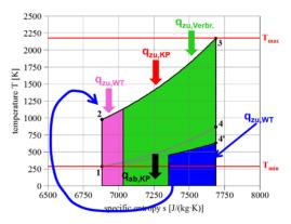
Fig. 12 – Joule cycle with recuperation of a part of heat at exhaust using a heat exchanger; this heat is induced in the next cycle before combustion.
