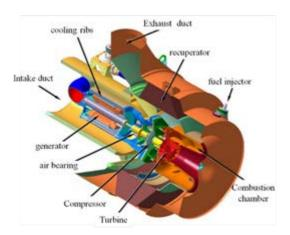
Fig. 7 – Schematic of a gas turbine with radial compressor and radial turbine (source: Capstone).
