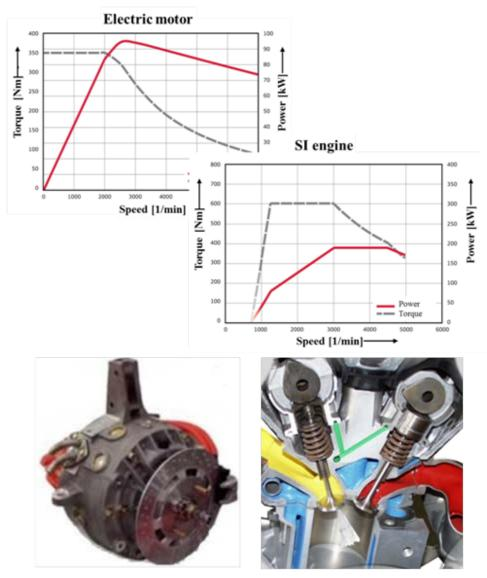
Fig. 1 – Typical torque/power curves for an electric motor and for an internal combustion engine for automobile propulsion.
