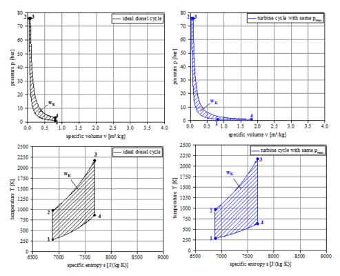
case is obvious. For a direct comparison the p,v- and the T,s- diagrams of both gas turbine variants and of the Diesel are superposed, as illustrated in Fig.11.
