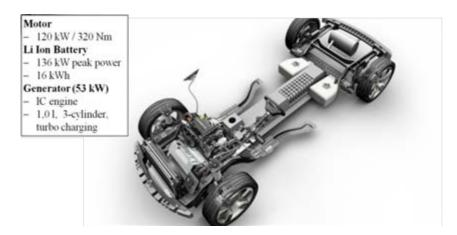
Fig. 2 – Four-stroke spark ignition engine as current generator for motor propulsion: Chevrolet E Flex Volt prototype (*source: General Motors*).
