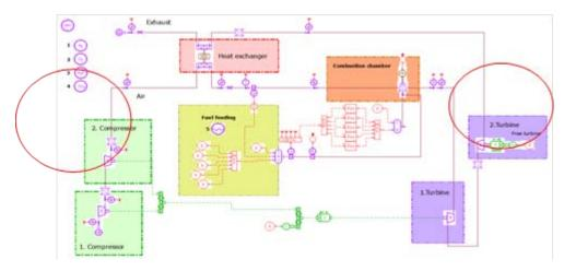
Fig. 14 – Configuration of the elements for the calculation of a gas turbine variant with heat recuperation using the Code AmeSim.
