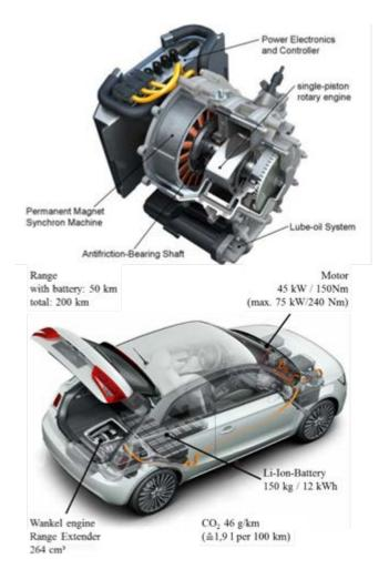
Fig. 5 - Wankel engine as current generator for motor propulsion: Audi e-tron (source: Audi).
