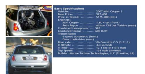
Fig. 8 - MINI Cooper S with propulsion by gas turbine (rear) and piston engine (front).
