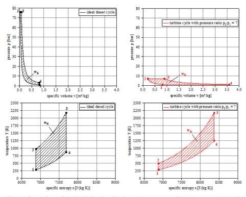
Fig. 9 – Comparison of the ideal Diesel and Joule cycles at same maximum temperature but with different maximum pressures.
