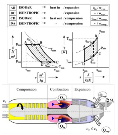
Fig. 6 – Ideal thermodynamic cycle (Joule process) and schematic of a turbomachine (gas turbine) with axial compressor and turbine [1].
