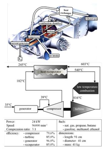
Fig. 13 – Schematic and function principle of a NoMac gas turbine.
