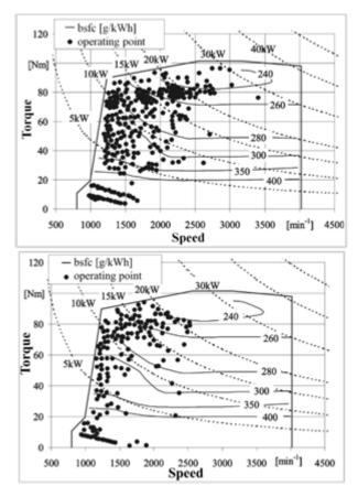
Fig. 3 – Operating domain of a middle-size car on country roads (left) and in an urban area (right) statistically [1].
