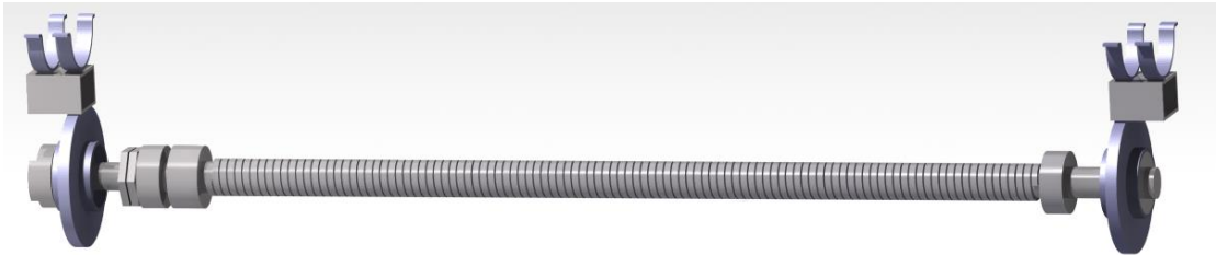
Figure 5: Assembling the screw with flanges, bars and collars
