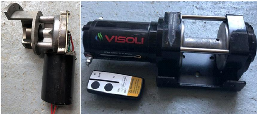
Figure 7: The 24 V electric motor and winch used to drive the immobilized bed care system
