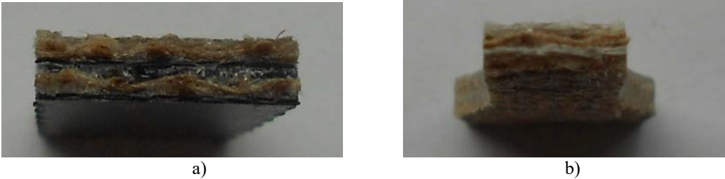
Figure 2. Sectional view of the composite hybrid C-Cnp (a) and the composite Hybrid S-Cnp (b)
