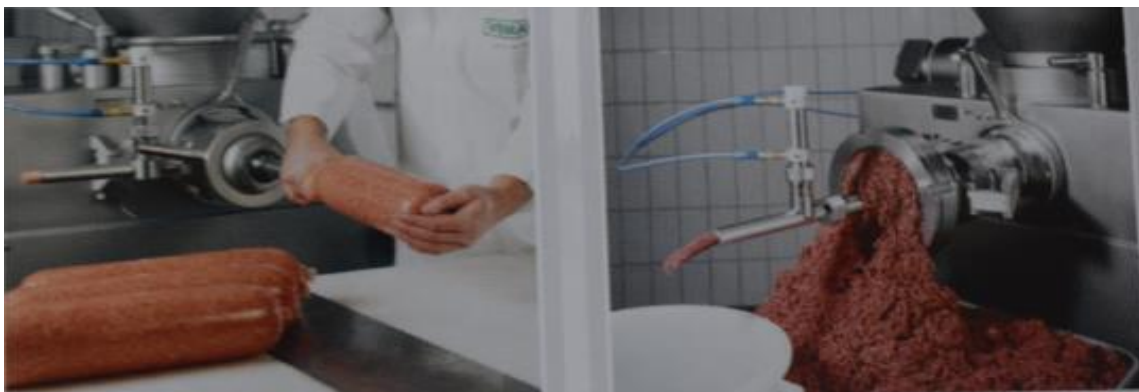
Fig.2 Filling the composition into the membrane
