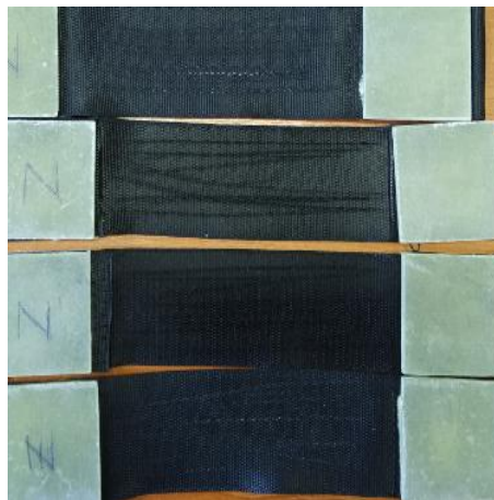
Figure 3: scratches on webbing
