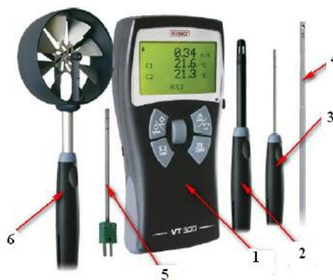
Figure 1. Thermo-hygro-anemometrul VT 300 ( www.kimo.fr )
