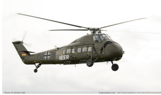
Figure 2: Sikorsky Aircraft S-58 (helicopter with a main rotor and a tail rotor) [5]
