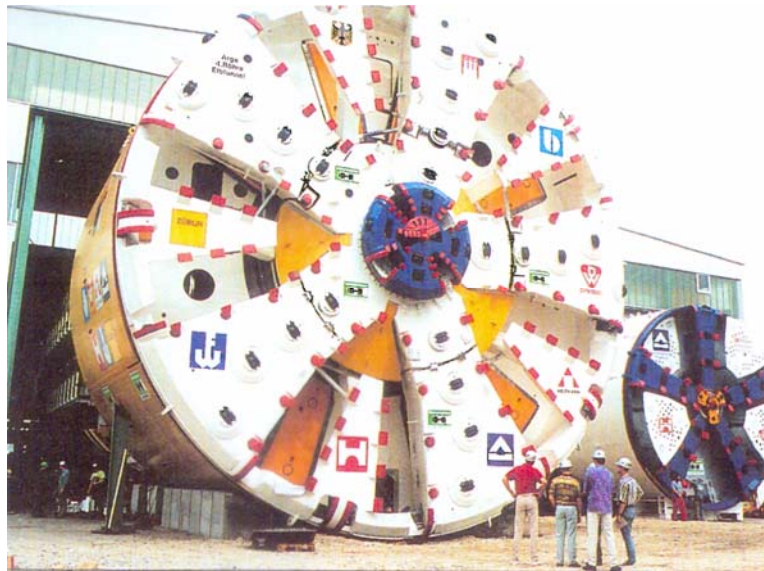
Fig.1 The biggest shield with total mill. Ø 14.2 meters in diameter. Subway in Berlin
