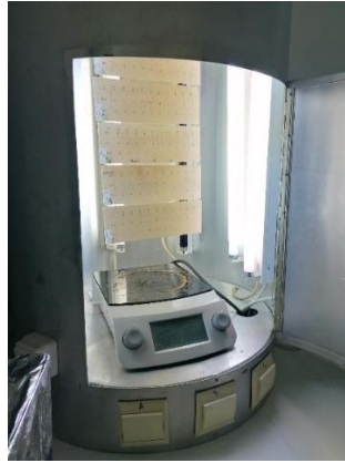
Figure 4: Photocatalytic reactor used for aging
