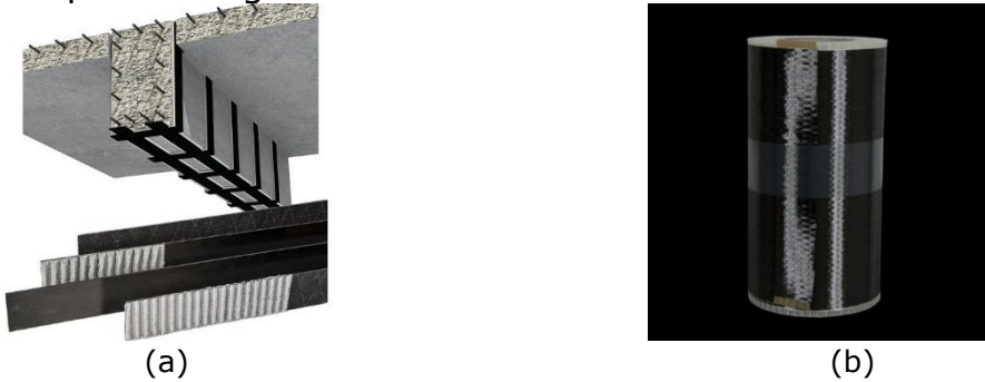
Figure 1: Materials used to strengthen the concrete beams: (a) CFRP pultruded plates used for beam reinforcement [17], and (b) woven sheets used for manufacturing of CFRP [21]
