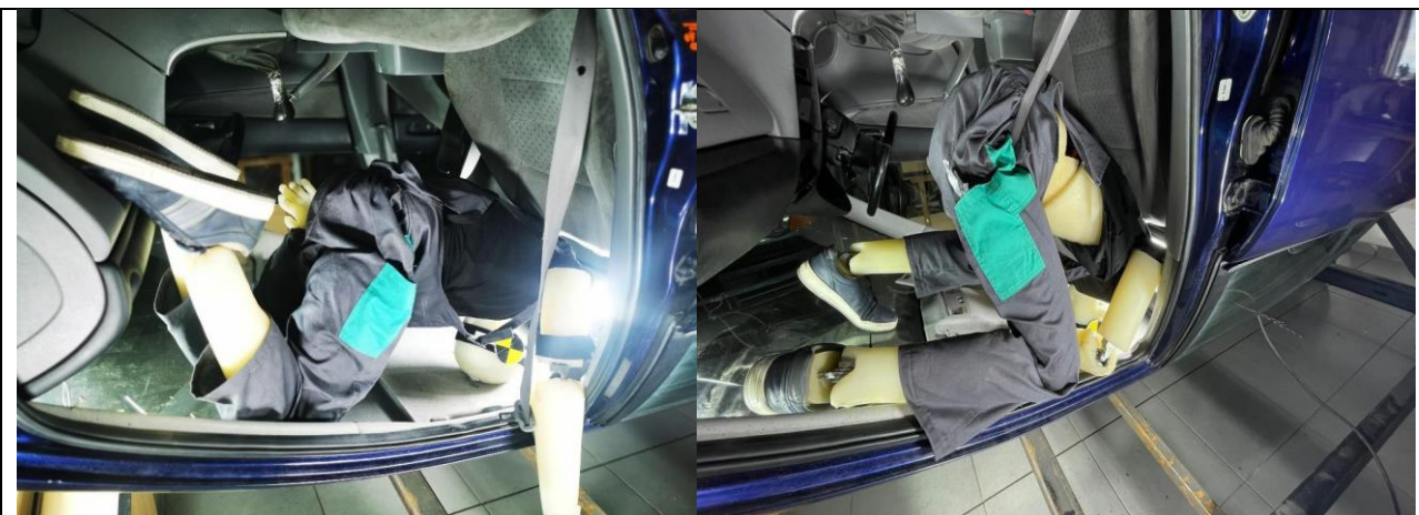
Fig. 2.2. The dummy in final position after the rolled over vehicle type tests
