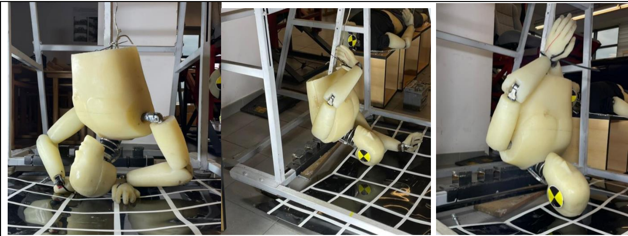
Fig. 2.1. The dummy position after the pendulum type tests
