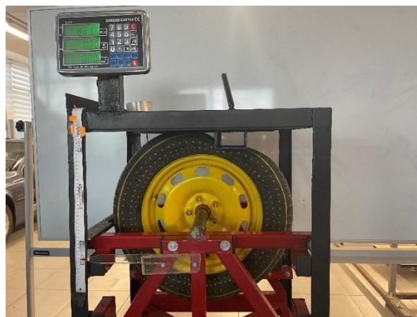
Figure 5: Tyre interaction with rectangular obstacle
