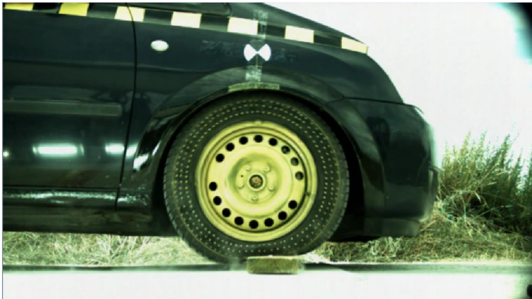
Figure 3. Maximum deformation of the tire in the first test
