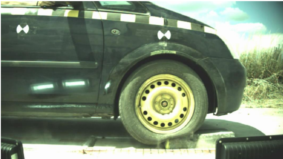
Figure 4. Maximum deformation of the tire in the tenth test
