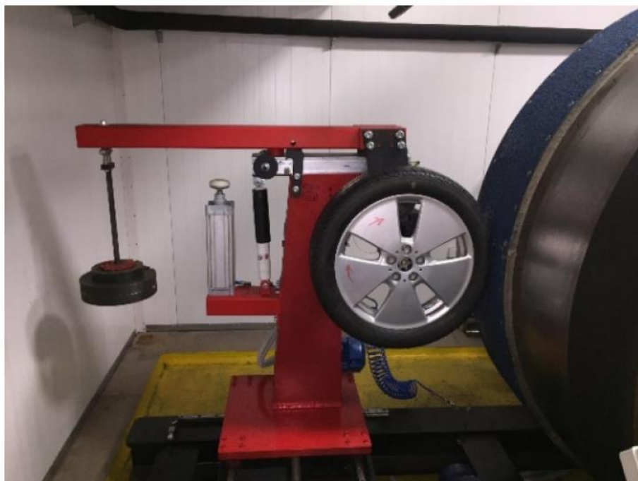
Figure 2. Stand for measuring rolling resistance
