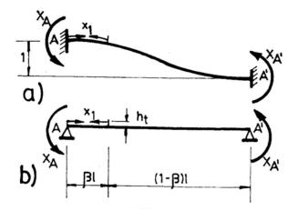
Fig. 4 – Prestressed Bar at One of Its Endsa). Deformed Axisb). Calculation System
