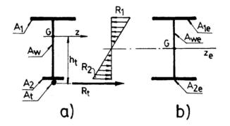
Fig. 2 a). Prestressed Section; b). Equivalent Section
