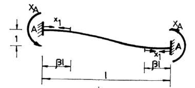
Fig. 5 – Deformed Axis of Prestressed Bar at Both Ends
