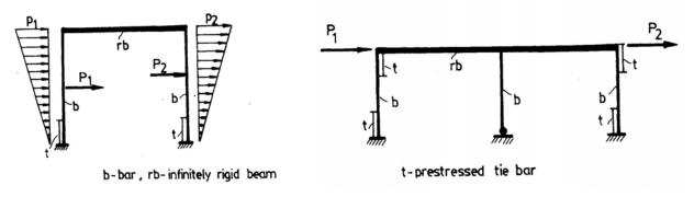
Fig. 1 - Examples of Prestressed Frames with the Infinitely Rigid Beam
