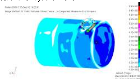
Figure 6: The maximum stress distribution on 5 layers for X axis, MAT-Roving material
