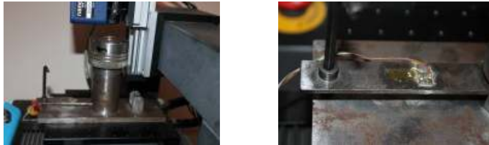
Figure 3: experimental device for the study of mechanical contacts under normal load by aid of laser profilometry and placement of the strain gauges used to evaluate applied forces
