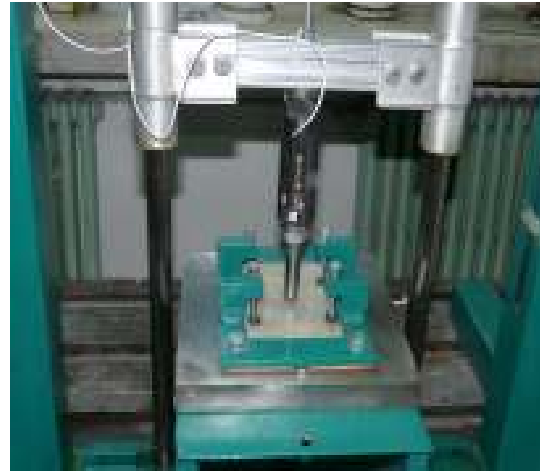
Figure 5 The positioning of the fixing screw the accelerometer
