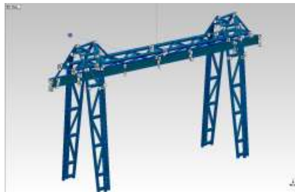
Fig. 8 Position of the measuring points on the crane's structure
