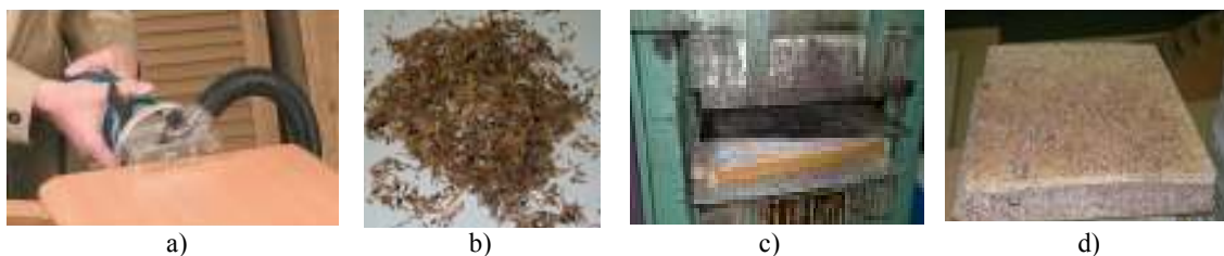
Figure 1: Technological steps of panels performed from acrylonitrile butadiene styrene (ABS) in laboratory conditions: a) ABS edge milling; b) ABS chips – residues; c) pressing mat chips; d) getting panels
